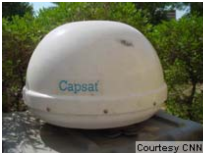
The dome cover of this vehicular Inmarsat antenna protects it from weather.
