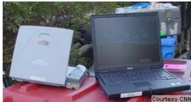
A laptop (right) can connect to a BGAN satellite antenna (left) to send data.
