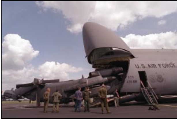
An MH-53J Pave Low helicopter is winched toward a C-5B Galaxy cargo plane at RAF Mildenhall, England.
