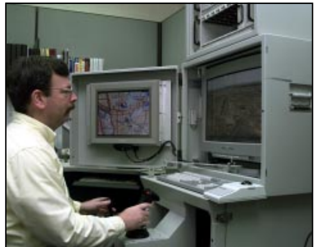
Computer-generated imagery system allows planners and crews to prepare flight routes and missions in three-dimensional target areas prior to mission execution.
