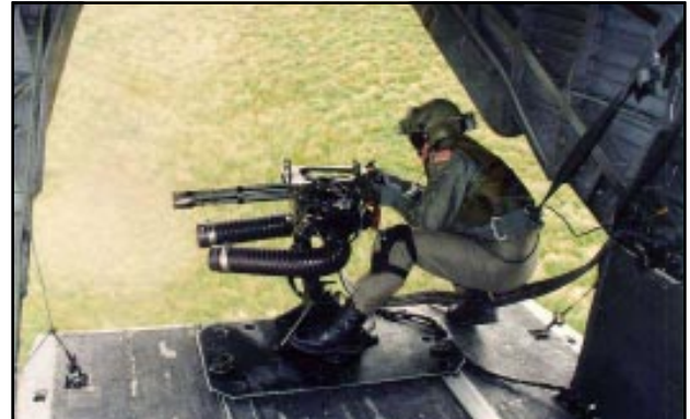
Tail gunner on MH-53J Pave Low helicopter employs suppressive fire support tactics with 7.62mm minigun.
